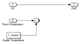
**6** Add labels to the signal lines to help trace model components to the equations and model requirements. Double-click above a signal line and enter a label.
