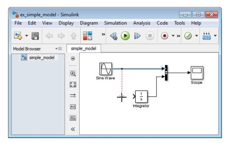
**3** Continue to drag the cursor to the Integrator input port, and then release the mouse button.
