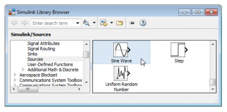
**3** Drag the Sine Wave block to the Simulink Editor. A copy of the Sine Wave block appears in your model with a text box for entering the value of the **Amplitude** parameter. In the text box enter **2**.
