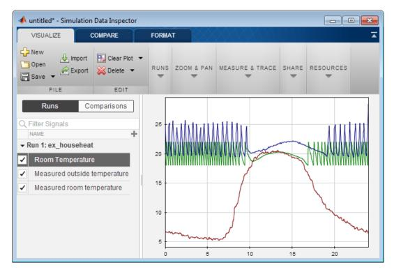
The top signal is the Measured Room Temperature. The middle signal is the simulated Room Temperature. The bottom signal is the Measured Outside Temperature.
