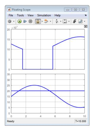
**Note:** If you get an error indicating Simulink cannot display a signal due to block reduction optimization, clear the **Block reduction** check box in the Configuration Parameters dialog box.
